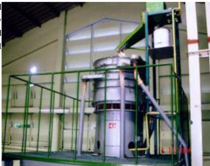
玻璃珠成套设备之筛分除磁设备 the sieving demagnetism for complete glass bead equipment
